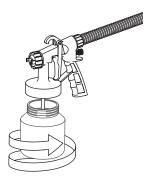
An airtight seal is essential for the correct operation of this spray gun. Before operating the unit please ensure that the paint container is securely fixed to the spray gun body and the gasket is in place.
